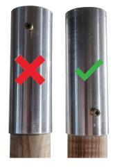
Once cured a 6 mm hole needs to be drilled in order to mount the locking pin. I recommend using a drill press. If you don't have one however carefully drilling with an electric hand drill is also viable. **Take utmost care to drill perpendicularly!** Drill 5-6 mm deep. Seat the brass locking pin by tapping it **lightly** in place with a wooden hammer. It should seat easily. If it doesn't widen the hole. Lock the pin in place using the provided philips head screw.
