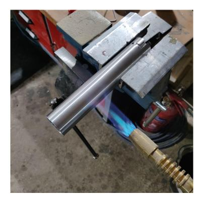
Have your partner insert the pole while keeping the flame on the aluminium tube. Excess wood will now burn off so be careful of the fumes. Check if the line you drew earlier has reached the edge of the tube. If so unclamp the tube and chill immediately. If not pull out the pole if possible heat and try again. If your pole can not be removed anymore - congratulations you just messed up. We will fix that later - for now just chill it down by dipping it in the bucket. Let it dry.
